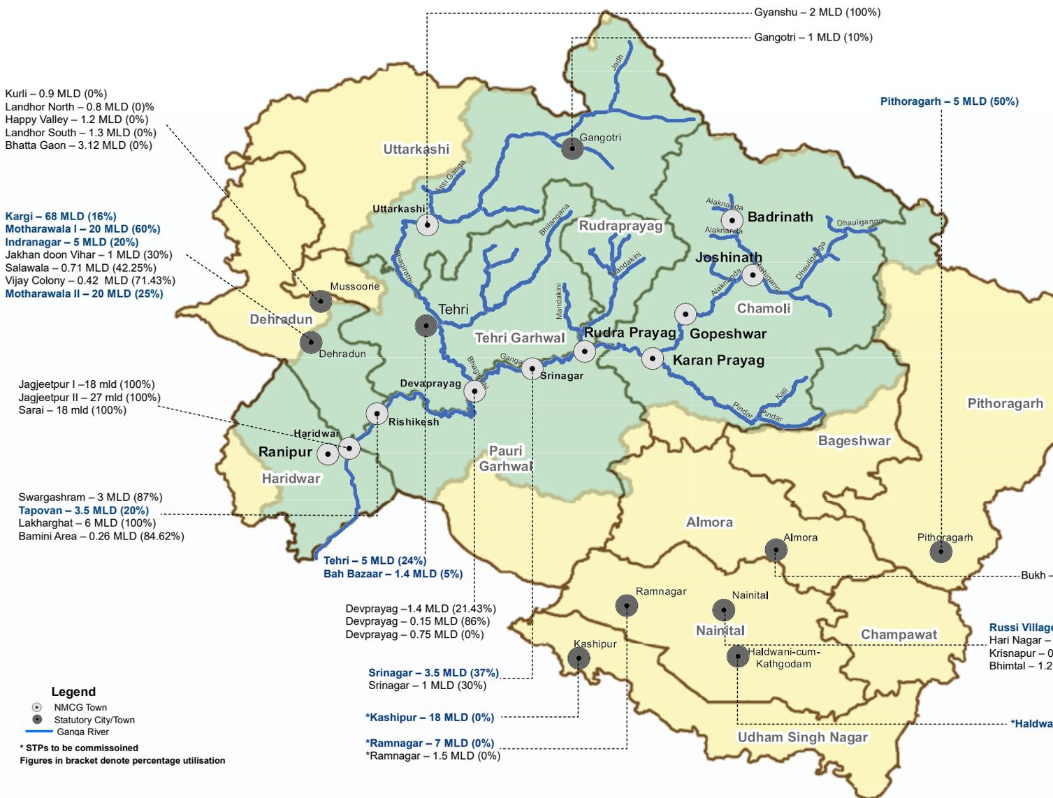
Note: STPs highlighted in blue shows higher potential for co-treatment of septage due to under utilized STPs.
